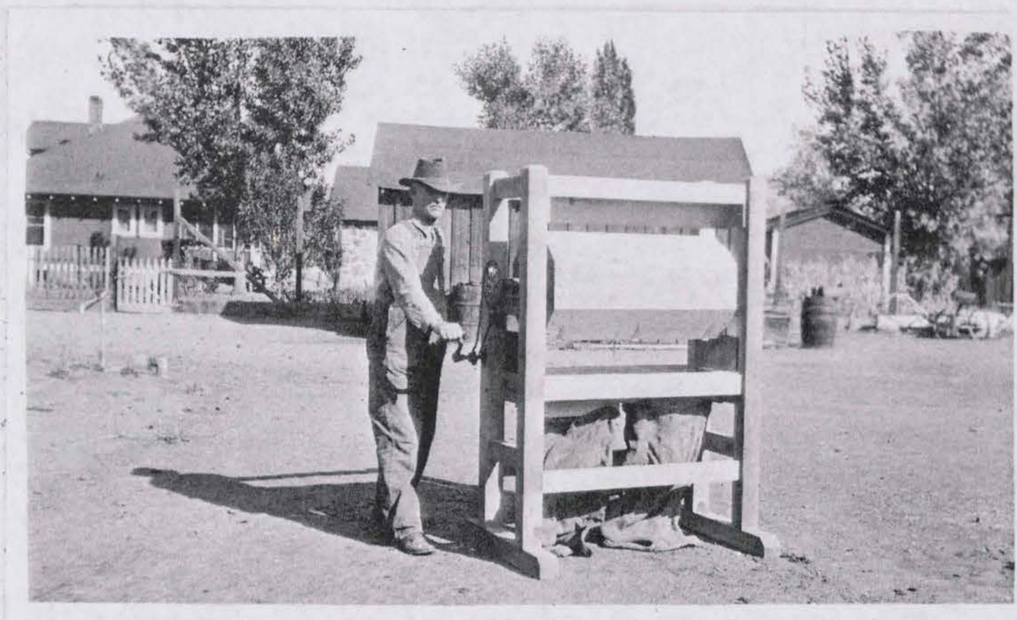
Fig. 2 Simple Machine For Dusting Seed Wheat With Copper Carbonate
