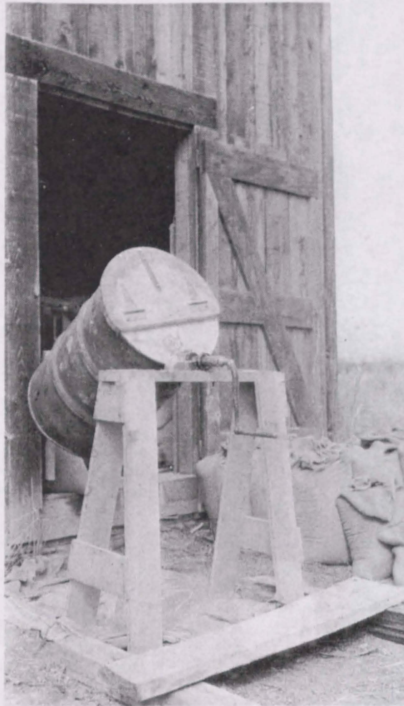
Figure 3. Type of home made dusting machine used. Objection is that of being hard to turn.
