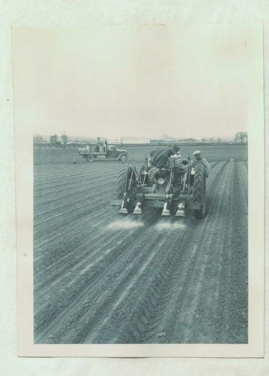
Weed burner being operated by a Nevada onion producer.
