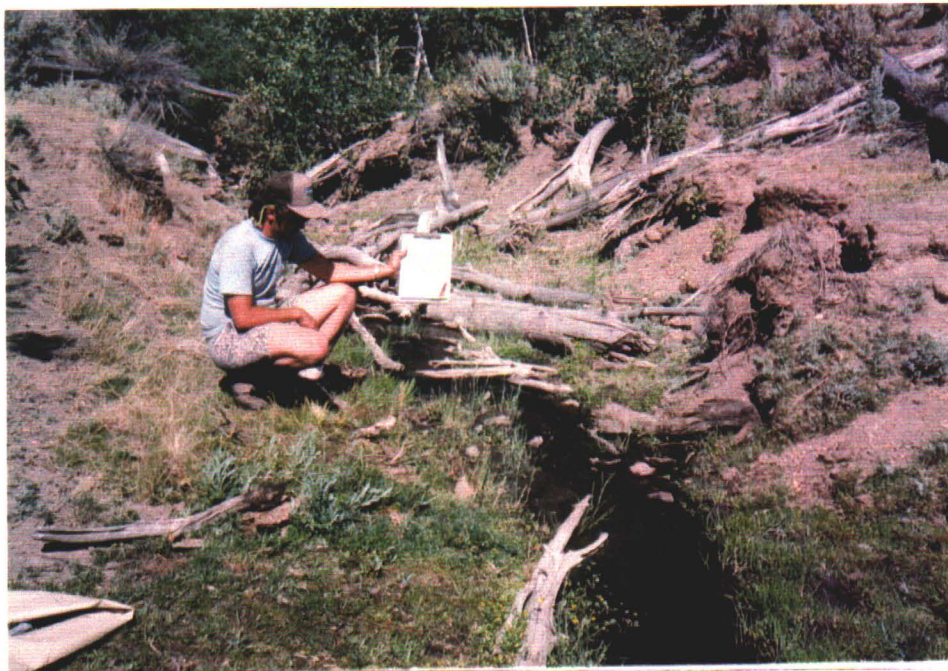
Sheep Creek, BLM stream survey station S-2. 7-22-92. Channel downcutting has led to draining of the historic floodplain and loss of the associated riparian zone including streamside aspen. Lack of floodplain development allows for concentration of flood flow energies, while the shallow channel profile and absence of any overhanging vegetation allows for excessive warming of the water column on hot summer days. Streambanks are mostly unstable and are only poorly vegetated.
