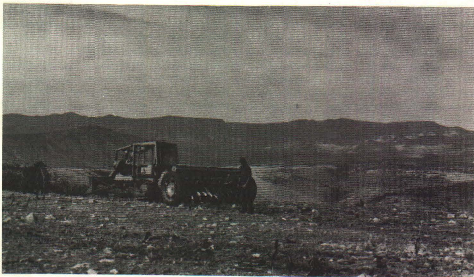
Rehabilitation efforts after a fire sometimes includes seeding. A rangeland drill like that shown drops the seed and immediately discs it into the ground.
