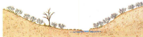
Stage 4: Channel widened enough to form a new stable channel and floodplain
