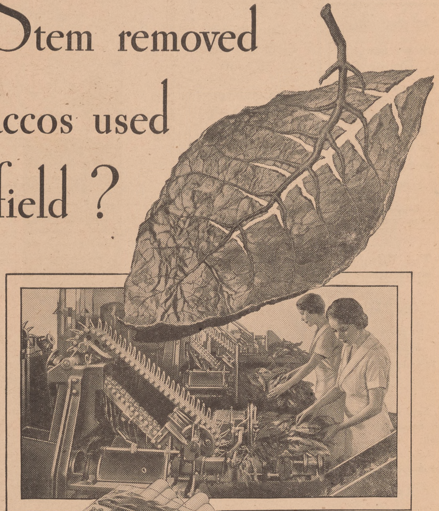
Tobacco used to be stemmed by hand—Now this machine stems 14,300 leaves every hour.
