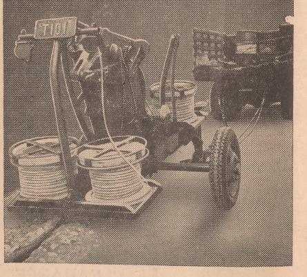
RURAL telephone wire-not in cables-can now go underground where bad weather and grass fires can't harm it.
