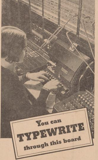
It looks like a telephone switchboard - actually it's a Teletypewriter exchange switchboard. Through such boards-located in 160 cities and townsalready more than 11,000 subscribers to Teletypewriter service are being inter-connected.
