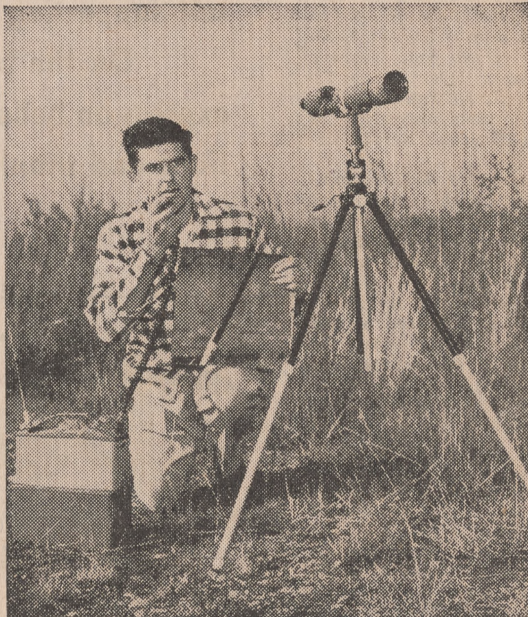
Here, Dick checks line-of-sight with a distant repeater station by mirror-flashing and confirms reception by portable radio. Using this technique, reflections of the sun's rays can be seen as far as 50 miles.
