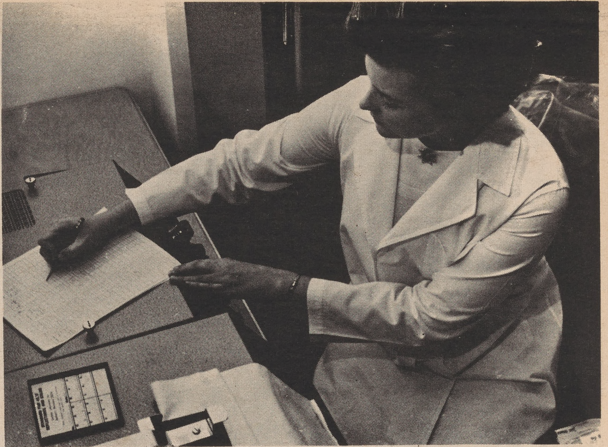
Barbara Ross, graduate student in home economics, is shown doing research for a six state regional textile project. Barbara is using the Gardner Color Difference Meter on samples of men's shirts to determine change in reflectance after a series of wear and laundering cycles.
