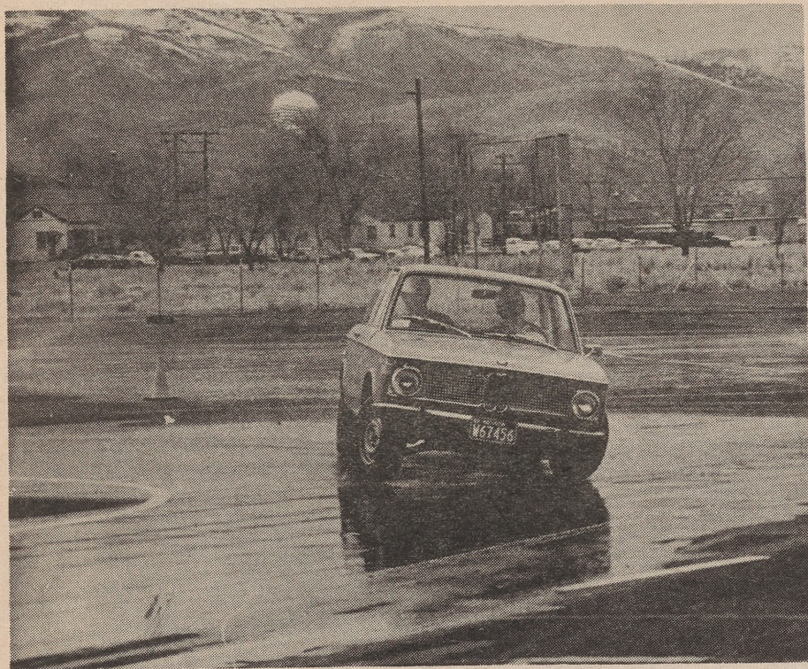
Driver Cartier turns the wheels in the direction of the skid to prevent a spin after sliding sideways off a curve.
